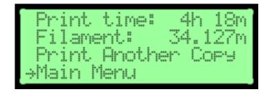
Figure 3.19: Print From SD Card Complete
