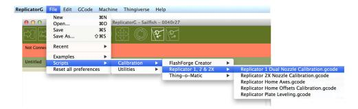
Figure 5.8: Nozzle Calibration Menu
