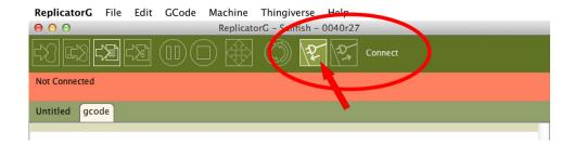
Figure 6.5: ReplicatorG: connect to your printer
