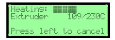
Figure 3.27: Extruder Heating
