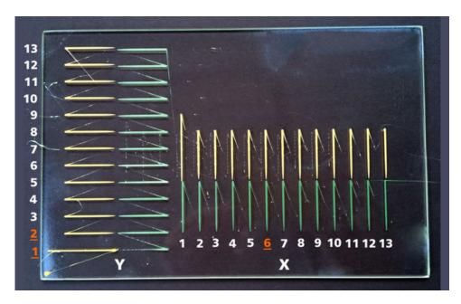
Figure 5.9: Nozzle Calibration Print
